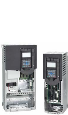
Wall Mount Frames 1...7 IP00/IP20, NEMA/UL Type Open Drive Includes a DC link choke on all Frames and internal brake transistor, standard on Frames 1...5, and optional on Frames 6 and 7.
