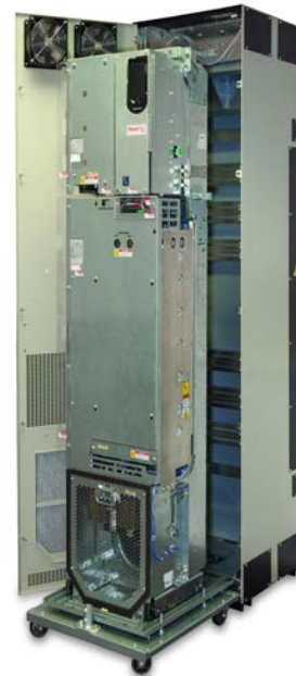
Roll-out Design (Frame 8 shown) A roll-out cart is required for Frames 8...10 drives and Frame 9...10 option bay chassis. The roll-out cart has an adjustable curb height of 0...182 mm (0...7.2 in.) and curb offset/reach of 0...114 mm (0...4.5 in.). See page 200 for information to order the roll-out cart.
