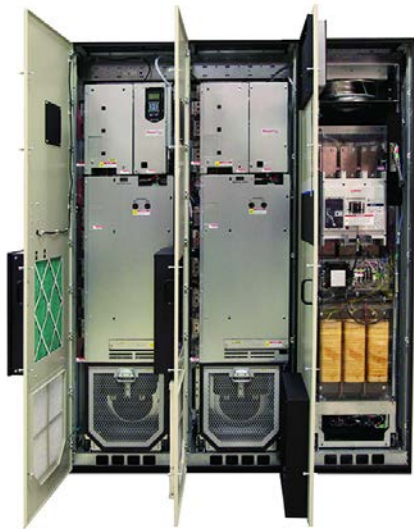
Floor Mount Frames 8...10 IP20, NEMA/UL Type 1 Drive with Options (2500 MCC style cabinet) Includes a DC link choke, integrated AC line fuses, roll-out design, and option bay for control/protection devices.
