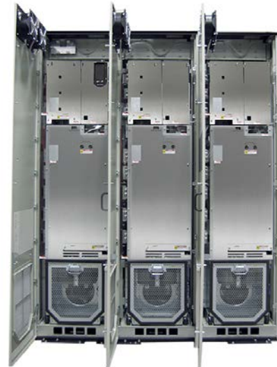
Floor Mount Frames 8...10 IP20, NEMA/UL Type 1 Drive (2500 MCC style cabinet) Includes a DC link choke, integrated AC line fuses, and roll-out design. Hood that is shown on top of cabinets is optional. To order the hood, see page 199 for information.
