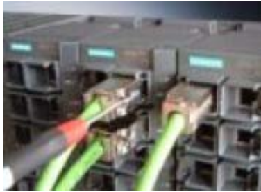
Figure A-4 Releasing the RJ-45 plug with a screwdriver (based on the example of the IE FC RJ-45 Plug 180)
